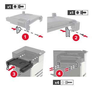
Attach the finisher to the printer.
