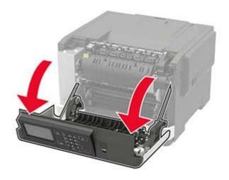
**2** Open the fuser access door, and then remove the jammed paper.
