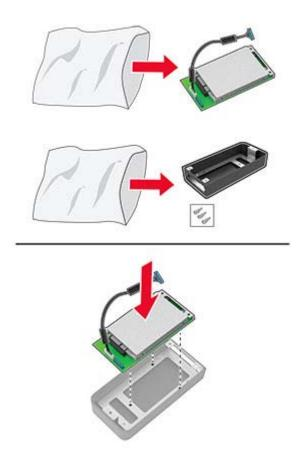
Attach the hard disk to the controller board access cover.
