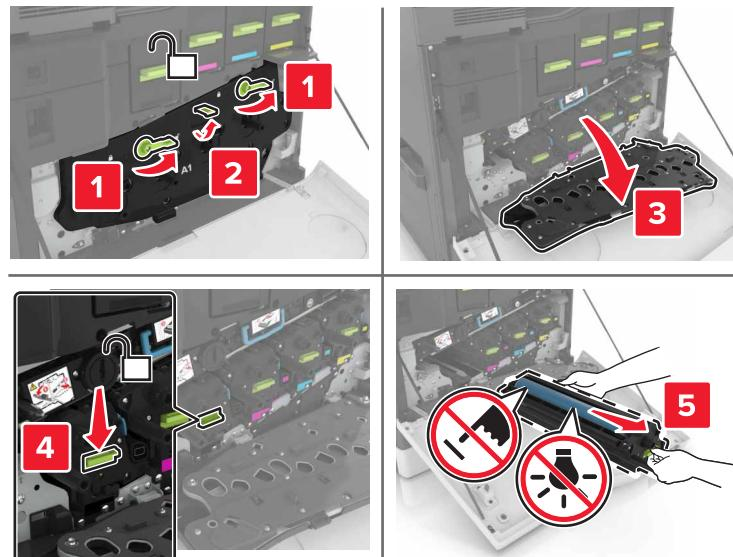
**4 移除感光鼓。**
