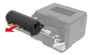
**3** Remove the used imaging unit.
