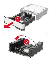
Remove the used pick roller assembly.
