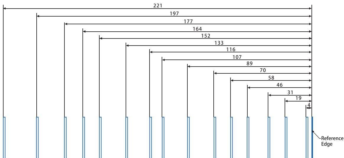
**Pola tulang rusuk untuk Lexmark C4150, C4342, C4352, CS720, CS725, CS727, CS728, CS730, CS735, CX725, CX727, CX730, CX735, XC4140, XC4150, XC4342, XC4352**
