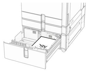
When loading letterhead for two-sided printing, load it facedown with the header toward the front of the tray.
