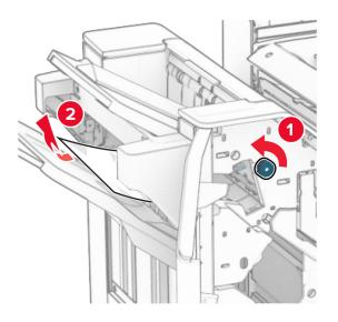
**10** Turn knob R2 counterclockwise, and then remove the jammed paper between doors N4 and N5.
