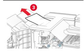
**12** Lift handle R4, turn knob R2 clockwise, and then remove the jammed paper.
