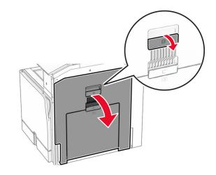
**12** Remove the jammed paper under the standard bin exit roller.
