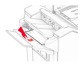
**2** Remove the jammed paper in the finisher standard bin.
