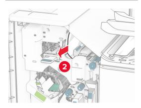
**10** Move handle R1 to the left, turn knob R2 counterclockwise, and then remove the jammed paper.
