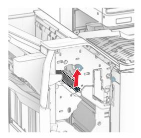
**9** Turn knob R3 counterclockwise, and then remove the jammed paper in bin 1.
