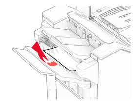
**2** Remove the jammed paper in the finisher standard bin.
