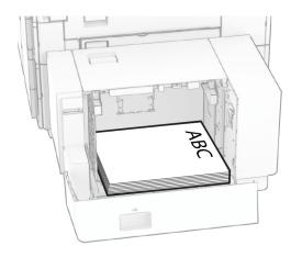
When loading a different paper size, make sure to adjust the guides. Do the following:
