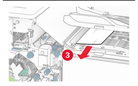
**11** Turn knob R5 counterclockwise, and then remove the jammed paper from the finisher standard bin.
