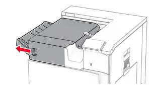
**3** Open door R1, and then rotate the knob R2 clockwise.
