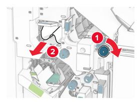
**11** Move handle R1 to the left, turn knob R2 counterclockwise, and then remove the jammed paper between doors N4 and N5.
